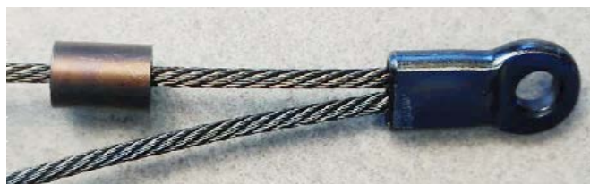
Picture 1: Examples of different color effects on the different materials rope, sleeve and eyelet
